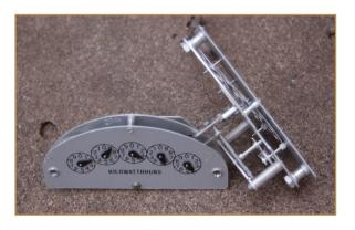
The electromechanical meter relies upon an intricate set of gears to accurately measure the amount of electricity used
